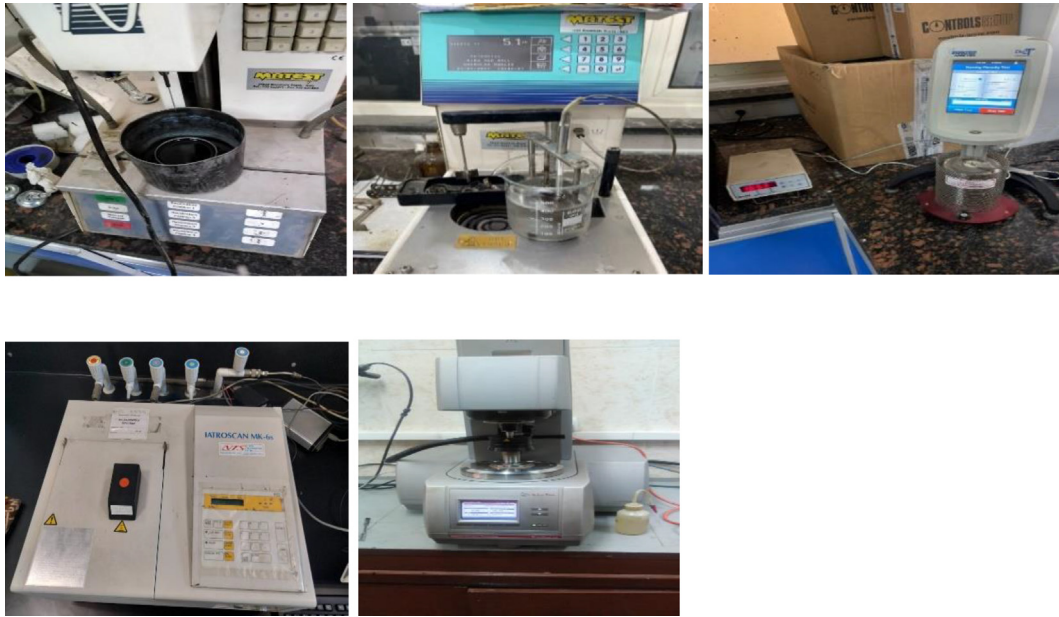
Fig. 4. (a) Penetration test, (b) softening point, (c) rotational viscometer, (d) ICP equipment, and (e) DSR test equipment.
