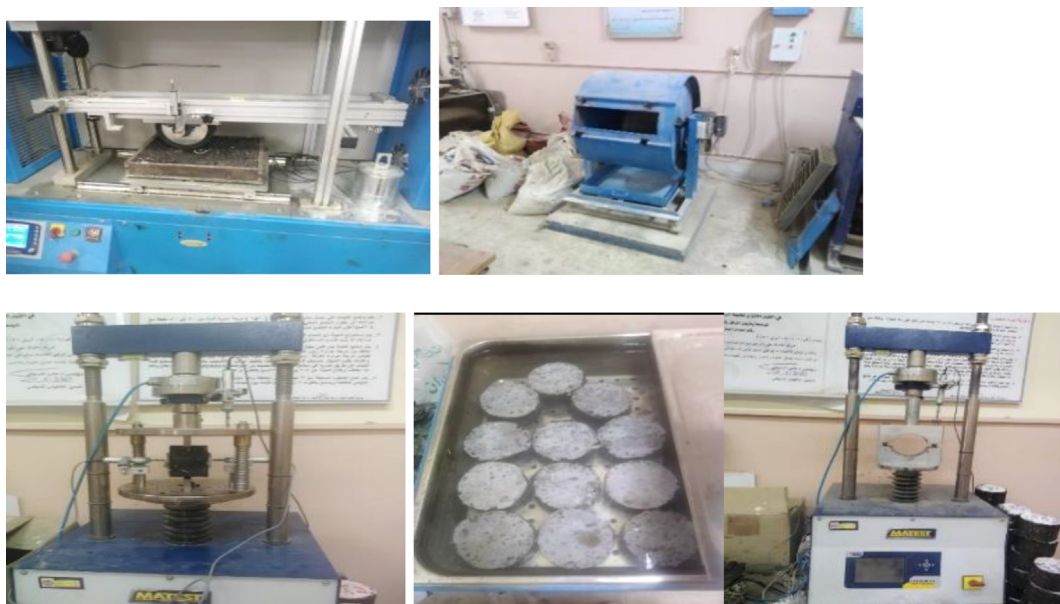
Fig. 14. (a) Hamburg wheel-tracking machine, (b) abrasion Los Angeles machine, (c) (IDT) strength tester machine and (d) Marshall testing machine.
